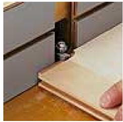
There are many times when I want to rout the *end* of a narrow work piece. The problem is the wood fibres on the back edge splinter as the bit exits the cut. Fortunately, all it takes to produce a crisp, clean cut is a simple backer block.
